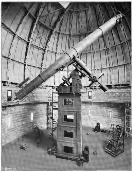
THE 40-INCH CLARK TELESCOPE OF THE YERKES OBSERVATORY MOUNTED BY WARNER & GRASEY
