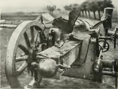
This fieldpiece was hit squarely on the muzzle by a shell. The rifling inside the barrel can be plainly seen
